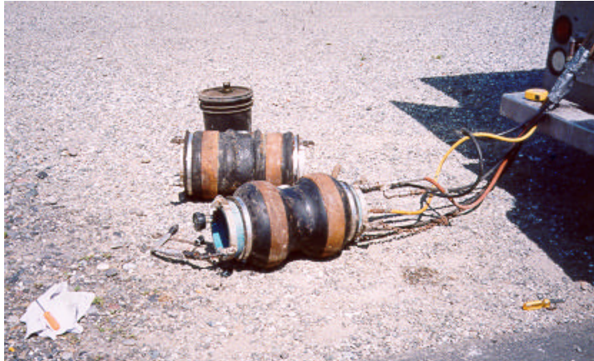
Figure 1. - Joint seal and pressure test device (August 2001). Photo by Jon Walter
